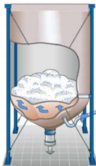
Bulk goods regain flow characteristics by means of the targeted introduction of Fluid-Ex®-system (Cross-section: Fluid-Ex®-system)
